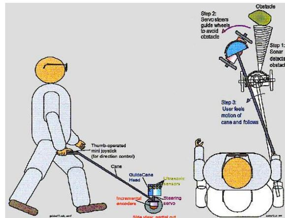
**Figure 1** Functional components of the Electronic Travelling Aid System [14]
