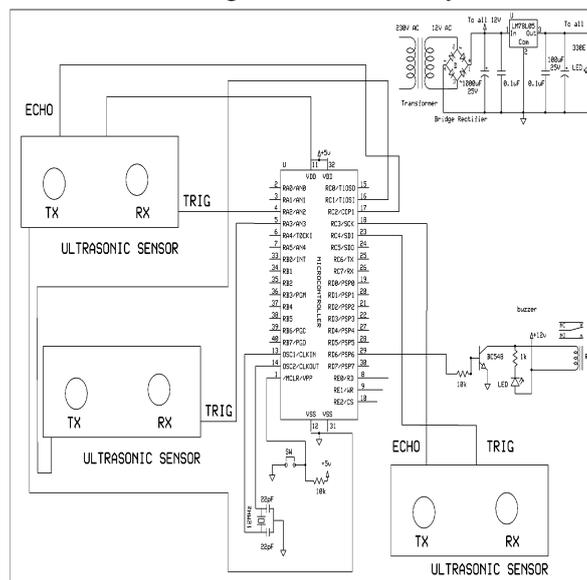
**Figure 2:** Circuit Diagram of Electronic Travelling Aid System
